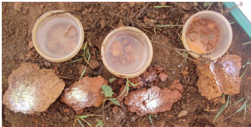
Figure 22. Photograph showing samples tested for soil pH (water) using the hand test kit. Samples on the left are A 1 and B 1 horizon samples showing acidic soil pH levels.
